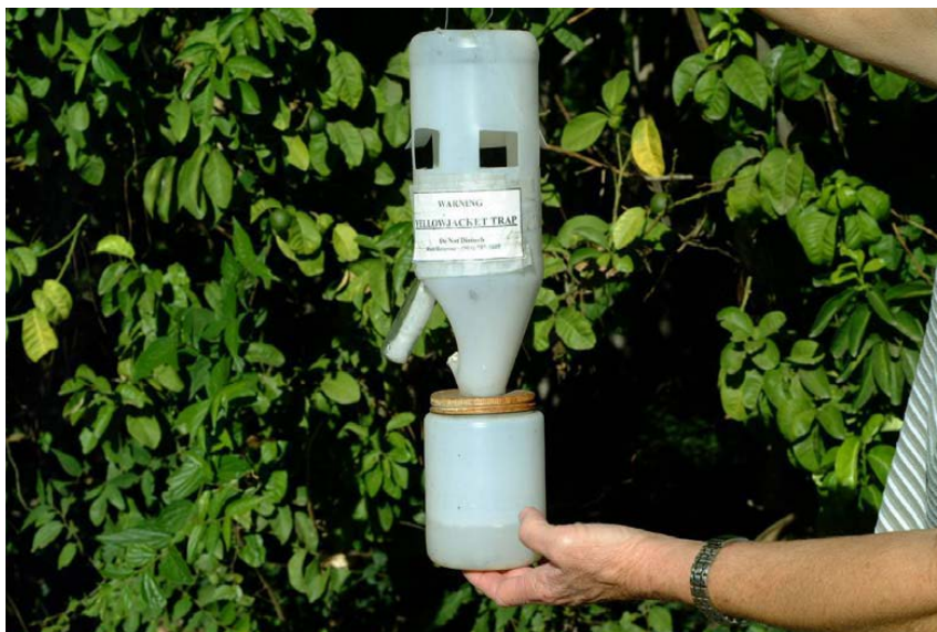
Fig. 2. The UCR-style trap with re-useable and interchangeable components.
