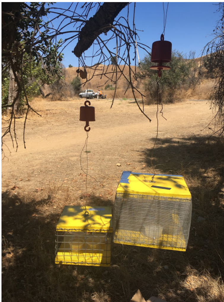
Fig. 24. A bait station (left) and an evaporation control station (right). Note the fine metal screen on the evaporation check station to prevent yellowjackets from foraging on the hydrogels.
